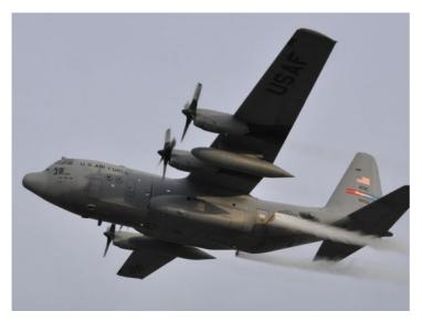
of harm's way by getting rid of the disease carrying vectors." The 910th's 757th Airlift six C-130H Squadron has Hercules aircraft complete with a modular aerial spray system, or MASS the Defense Department's only aerial spray maintenance flight. The products they carry in their aerial spray tanks vary depending mission, said maintenance chief
